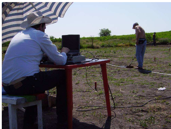
Scanning of an archaeological site by GPR by the team of archaeo- geophysical lab.
